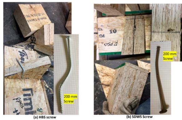
Figure 18. Failure mode of Connection-A in shear loading: (a) HBS screw; (b) SDWS screw.
