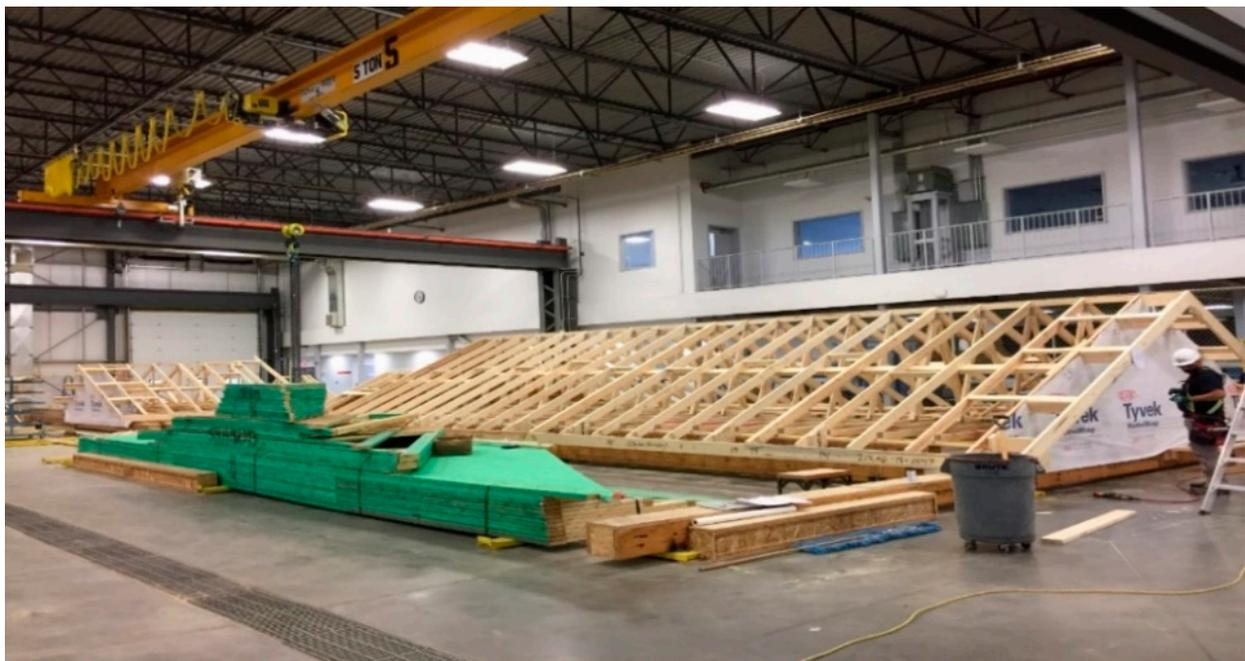
**Figure 2.** A roof production line (courtesy of ACQBUILT, Inc., Edmonton, AB, Canada) [2].
