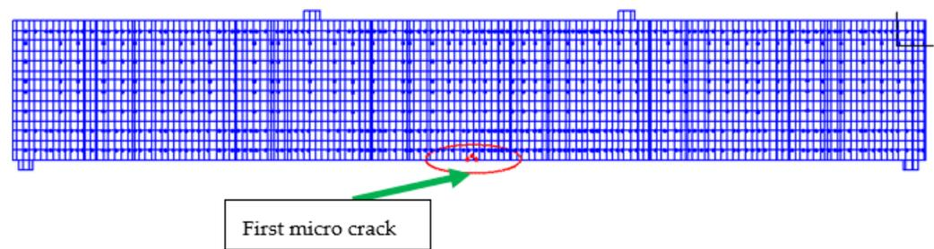
Figure 12. First cracks of specimen S0.
