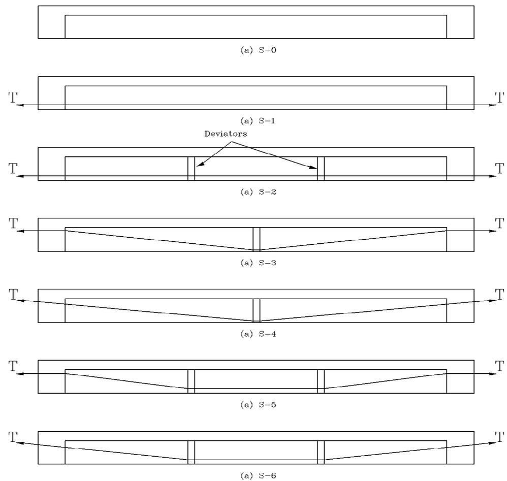
**Figure 2.** Several techniques for the external pre-stressing of simple beams.
