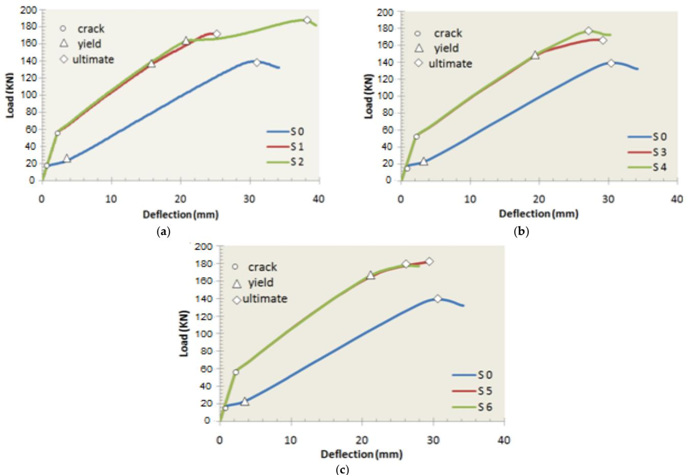
**Figure 15.** Load–displacement relation of all specimens: (a) straight-line tendons (S0 with S1 and S2); (b) V-shaped tendons (S0 with S3 and S4); (c) U-shaped tendons (S0 with S5 and S6).
