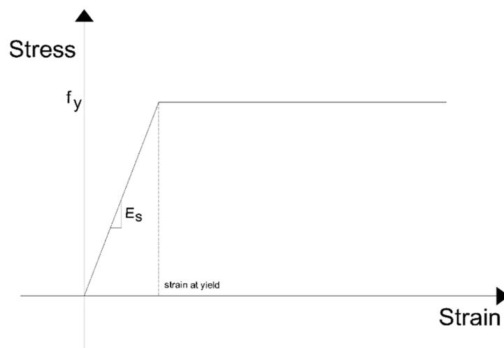
**Figure 7.** Constitutive law for steel reinforcement (Adapted from Refs. [19,20]).
