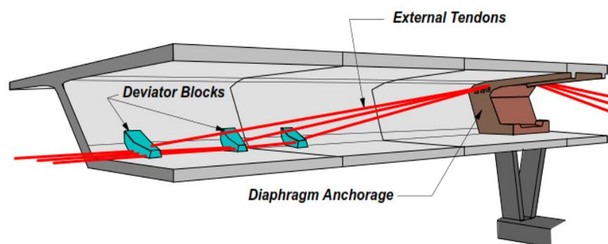
**Figure 1.** Layout of an externally post-tensioned box girder bridge.
