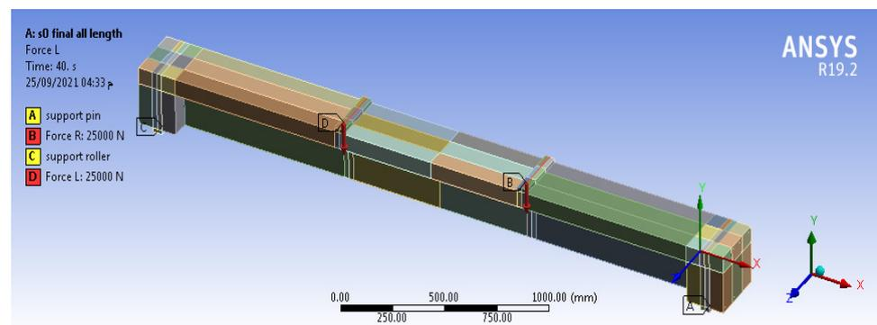
Figure 5. The FE applied loads for specimens.
