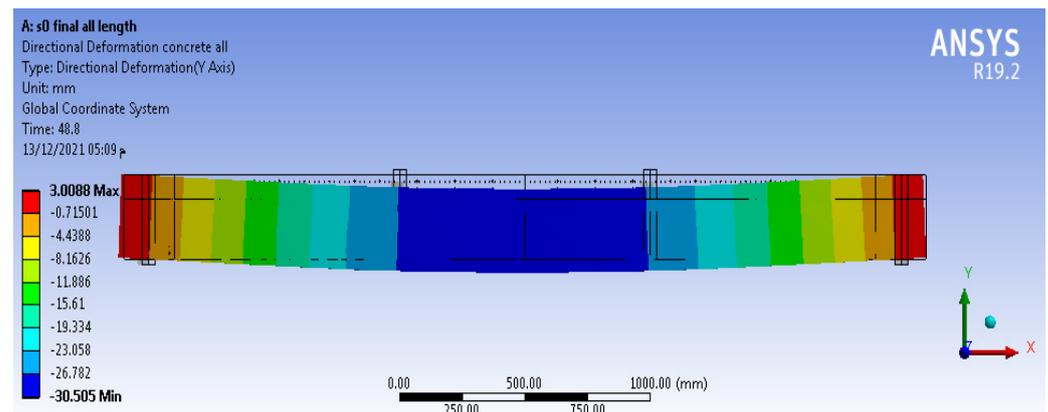
Figure 14. Vertical deflection at the failure of specimen S0.
