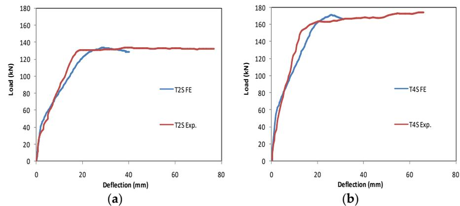
**Figure 10.** Load–displacement relation for laboratory tests (Adapted from Ref. [26]). versus FE tests: (a) Beam T2S; (b) Beam T4S.
