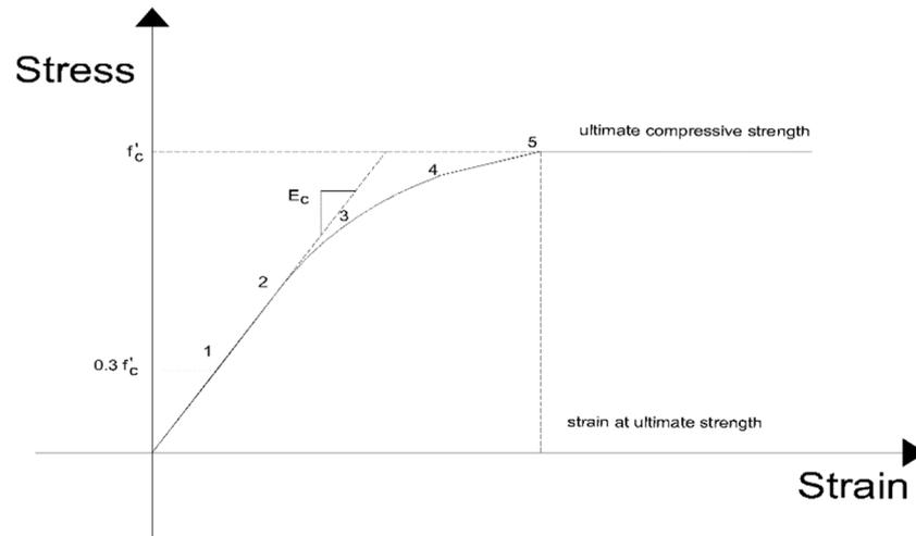
**Figure 6.** Simplified compressive Uniaxial stress-strain curve for concrete (Adapted from Refs. [19,20]).
