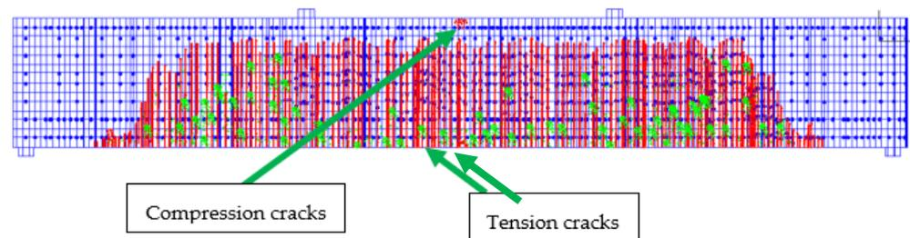
Figure 13. Cracks at failure of specimen S0.
