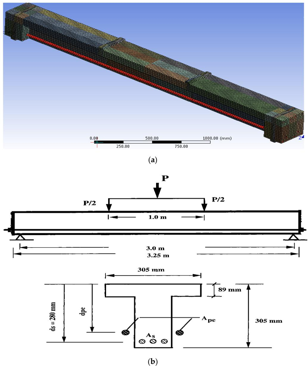
**Figure 9.** Loading method and external tendon profile: (a) FE; (b) experimental (Adapted from Ref. [26]).
