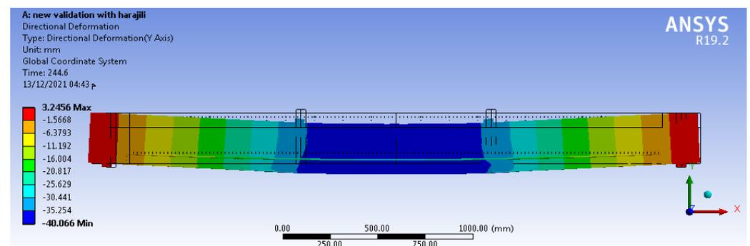
**Figure 11.** Vertical deflection at failure of specimen T2S.
