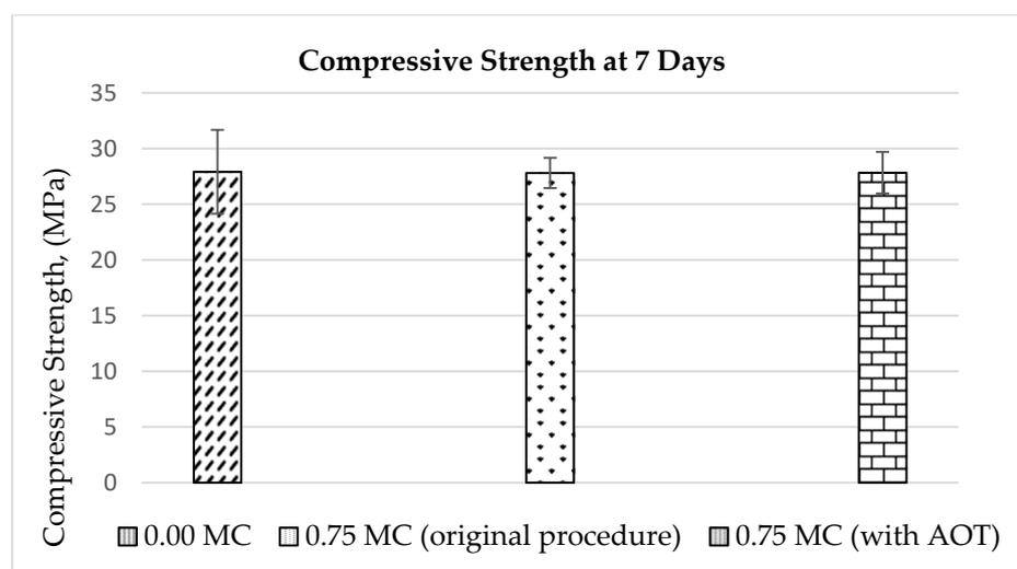
**Figure 4.** Compressive strength versus microcapsule concentration at 7 curing days (Error bars = standard deviation).
