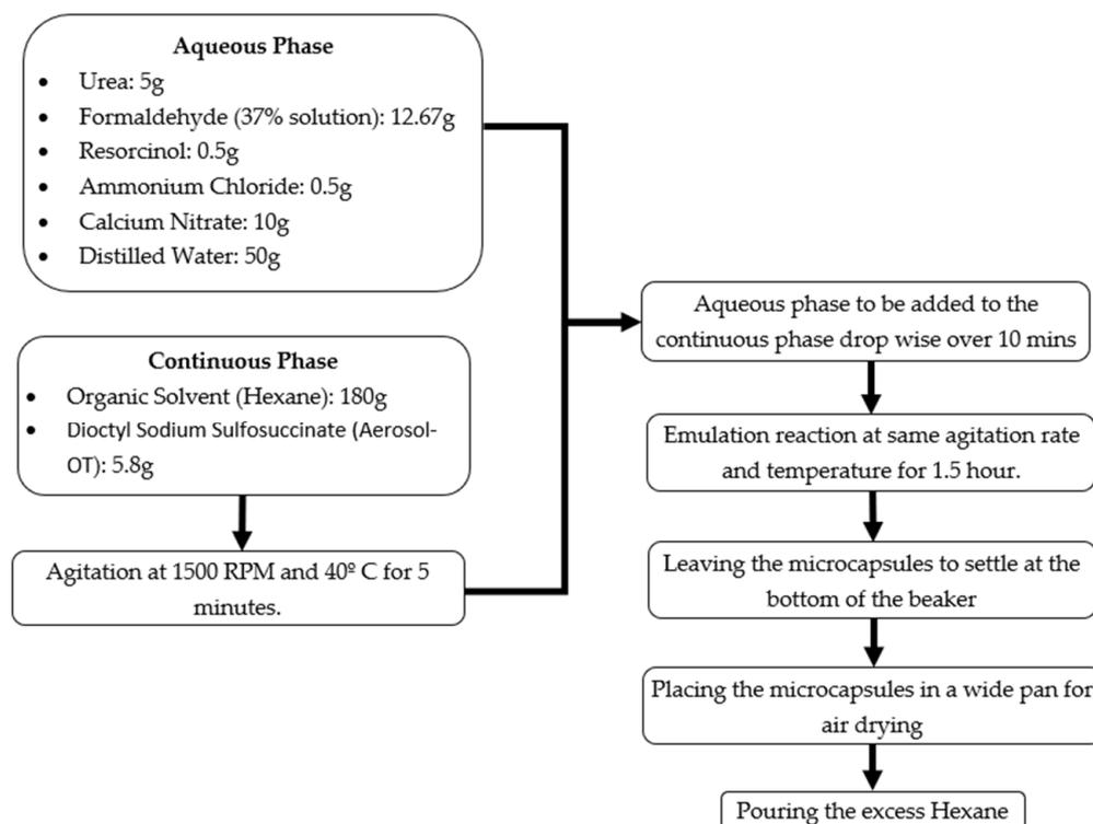
**Figure 1.** Microcapsule preparation method schematic illustration.
