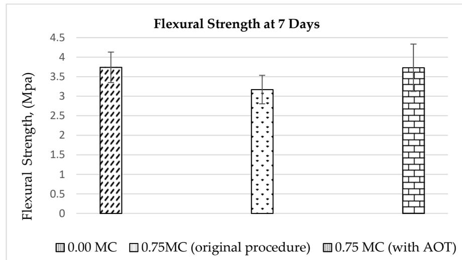
**Figure 5.** Mortar flexural strength versus microcapsule concentration at 7 curing days (Error bars = standard deviation).
