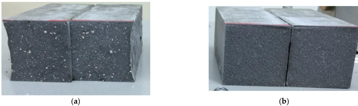
**Figure 6.** Samples after flexural breaking (a) microcapsules prepared using the original procedure and (b) microcapsules prepared using AOT.
