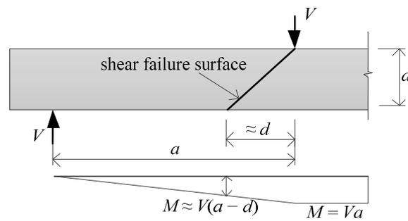
**Figure 2.** Critical section in ACI model.
