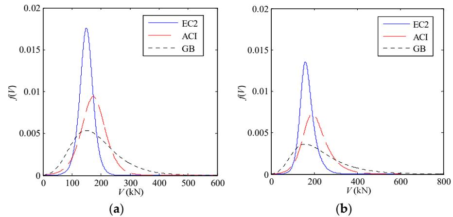
**Figure 7.** Comparison of the PDFs of shear capacity by different models. (a) PDFs of  $V_b$ . (b) PDFs of  $V_s$ .
