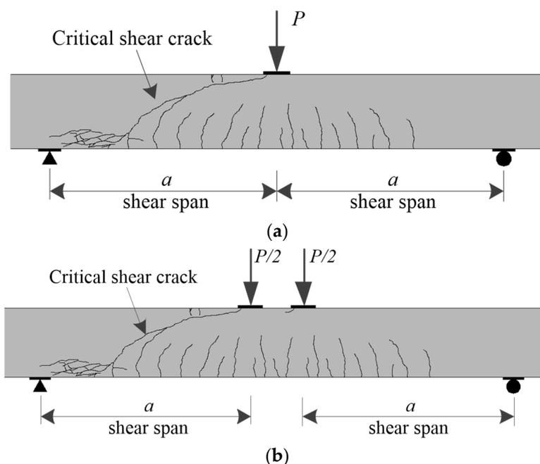
**Figure 1.** Typical shear test for RC beams. (a) three-point symmetrical loading. (b) Four-point symmetrical loading.
