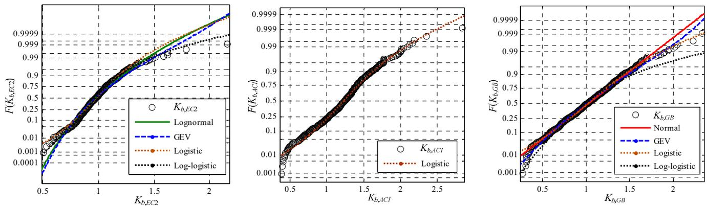
**Figure 4.** Fitting of the model uncertainty  $K_{pb}$  by the distributions accepted by KS test.
