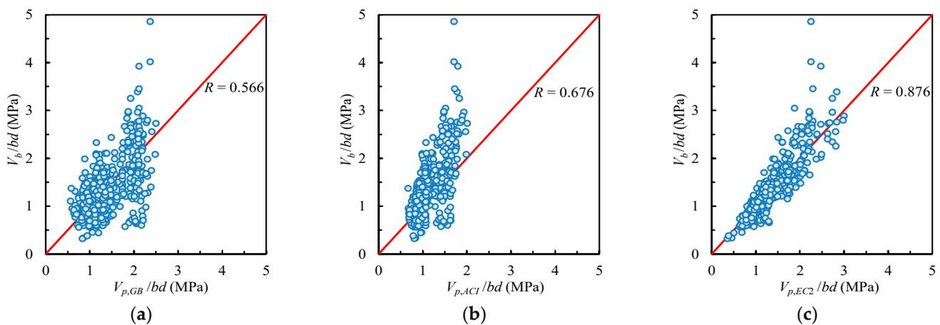
**Figure 3.** Comparison of model predictions with test results. (a) EC2. (b) ACI. (c) GB.
