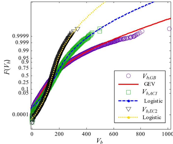
**Figure 5.** Distribution fitting of the beam capacity  $V_b$ .
