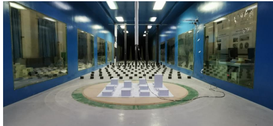
Figure 5. Wind tunnel test site layout.
