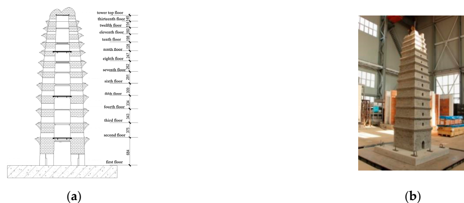
Figure 3. Tower dimensions and overall model. (a) Tower size; (b) Overall model.
