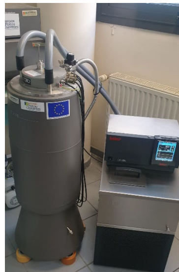
Figure 2. Image of the BT 2.15 Calvet calorimeter.
