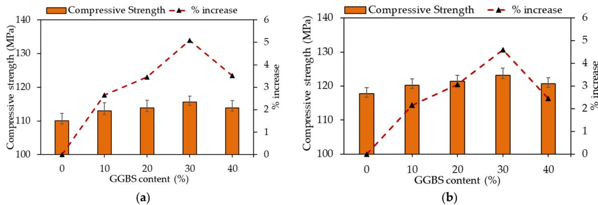
**Figure 6.** Compression test results of RPC mixes: (a) non-fibrous mixes; (b) fibrous mixes.
