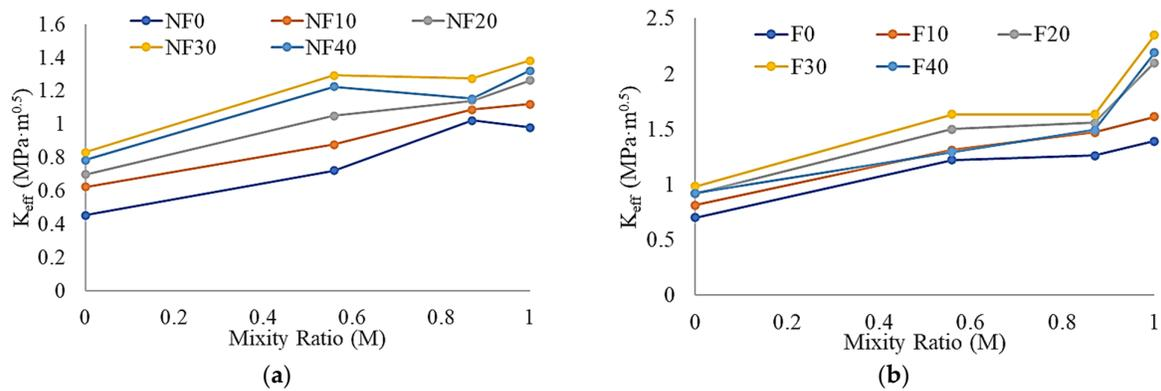
**Figure 12.** Effect of loading mode on fracture toughness of RPC mixes: (a) mixture ratio vs. effective fracture toughness for non-fibrous mixes; (b) mixture ratio vs. effective fracture toughness for fibrous mixes.
