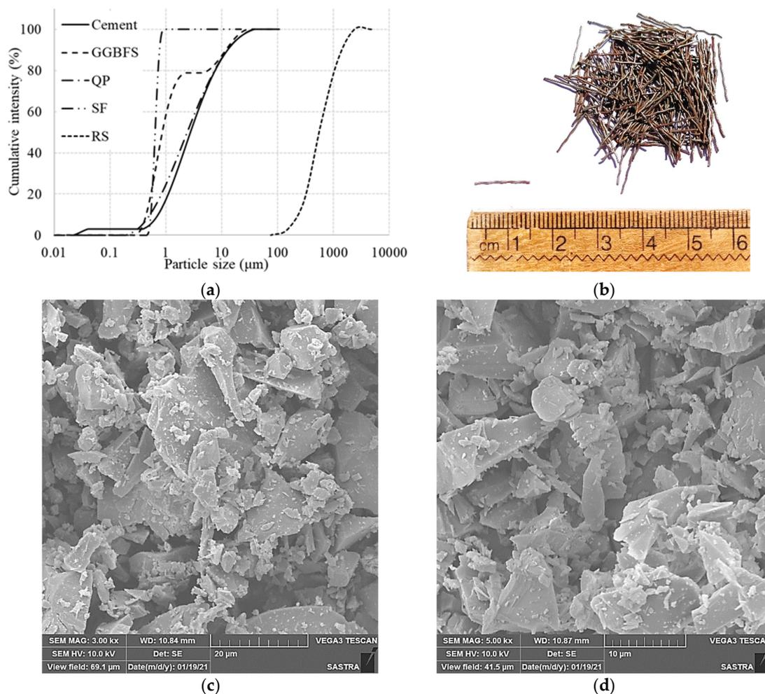
**Figure 1.** Material properties: (a) particle size distribution of constituent powders; (b) profile of crimped steel fibres; (c) SEM micrograph of GGBS at 3000× magnification; (d) SEM micrograph of GGBS at 5000× magnification.
