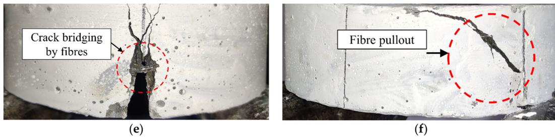
**Figure 13.** Typical failure patterns of tested specimens: (a) non-fibrous specimens at  $\beta = 0^\circ$ ; (b) non-fibrous specimens at  $\beta = 20^\circ$ ; (c) non-fibrous specimens at  $\beta = 50^\circ$ ; (d) non-fibrous specimens at  $\beta = 63^\circ$ ; (e) fibrous specimens at  $\beta = 0^\circ$ ; (f) fibrous specimen at mixed modes and pure mode III.
