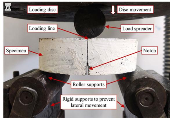
**Figure 4.** Experimental setup: (a) pure mode I ( $\beta = 0^\circ$ ) specimen; (b) mixed mode I/III ( $\beta = 20^\circ$ ) specimen; (c) mixed mode I/III ( $\beta = 50^\circ$ ) specimen; (d) pure mode III ( $\beta = 63^\circ$ ) specimen; (e) experimental setup for testing ENDB specimens.
