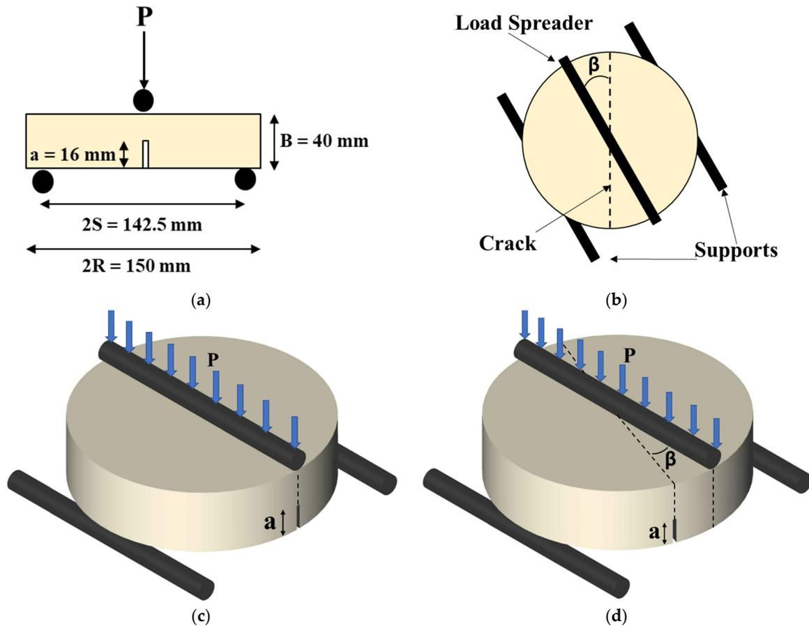
**Figure 3.** Scheme of experimental setup: (a) geometry of ENDB specimens; (b) arrangement of supports and load spreader; (c) scheme of loading ENDB specimens for pure mode I; (d) scheme of loading ENDB specimens for pure mode III and mixed modes I/III.
