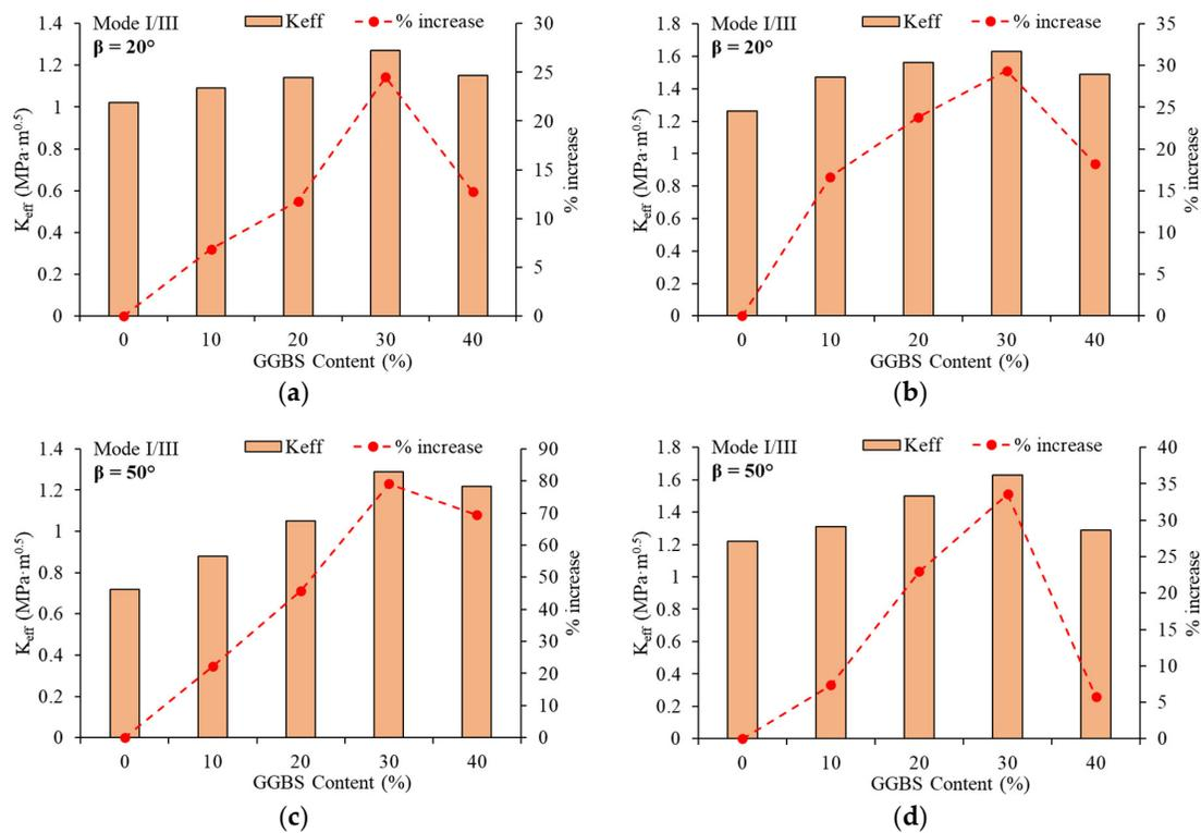
**Figure 10.** Effect of GGBS addition on mixed mode fracture toughness of RPC mixes: (a) non-fibrous mixes at  $\beta = 20^\circ$ ; (b) fibrous mixes at  $\beta = 20^\circ$ ; (c) non-fibrous mixes at  $\beta = 50^\circ$ ; (d) fibrous mixes at  $\beta = 50^\circ$ .
