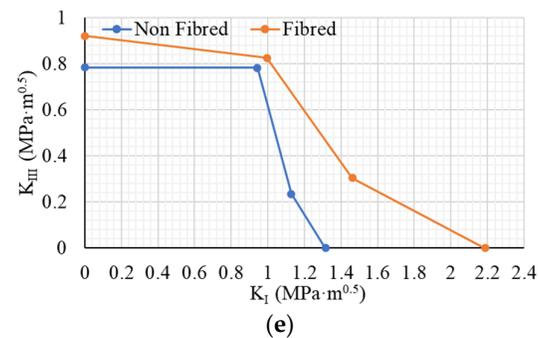
**Figure 11.** Effect of addition of fibres on fracture toughness of RPC mixes: (a) mixes with 0% GGBS; (b) mixes with 10% GGBS; (c) mixes with 20% GGBS; (d) mixes with 30% GGBS; (e) mixes with 40% GGBS.
