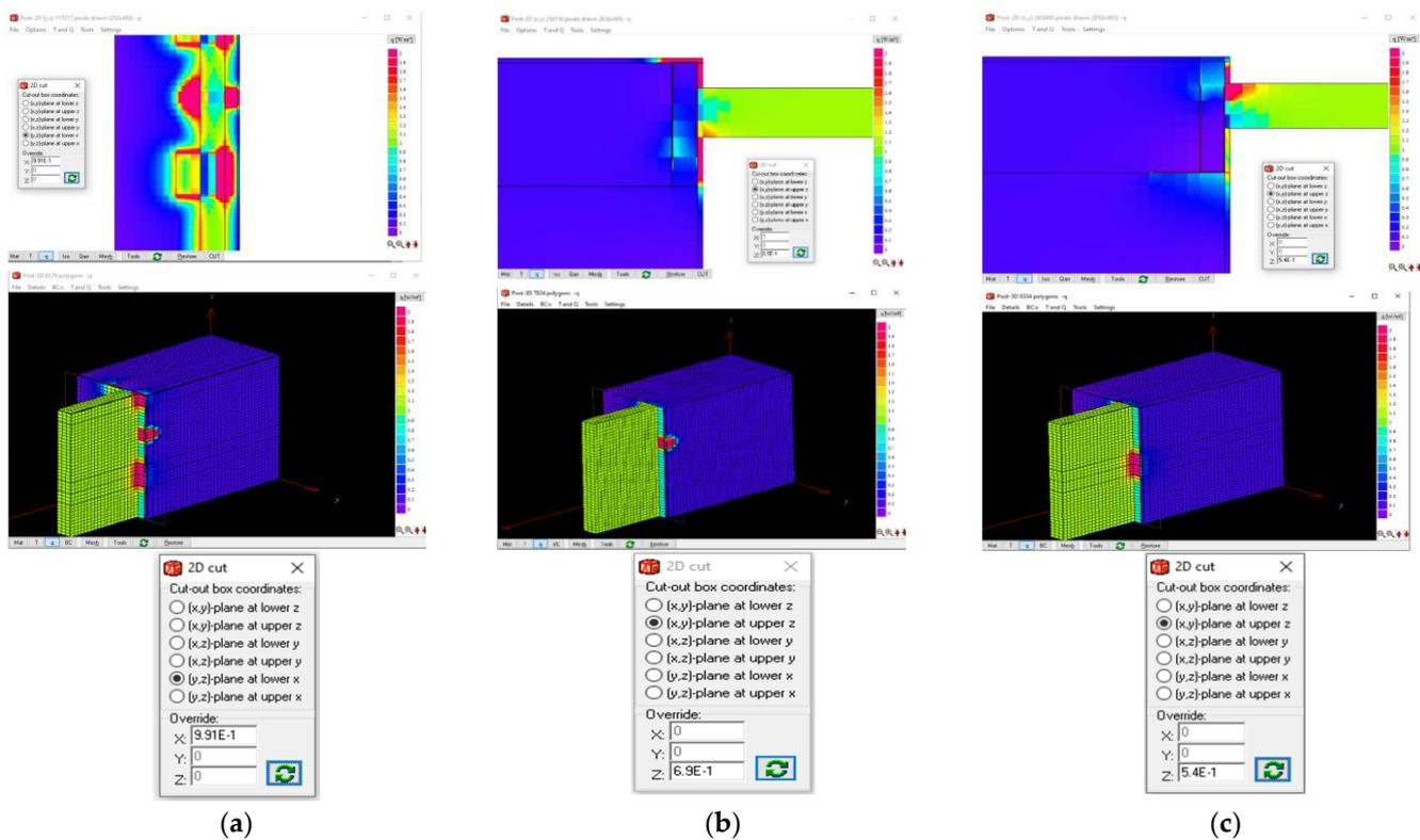
**Figure 11.** Intensity of heat flows in the cross-section of fasteners: (a) set of fasteners: corner fastener CL, interconnect fastener EL, and window frame fastener W; (b) separate W fastener; (c) separate EL fastener.
