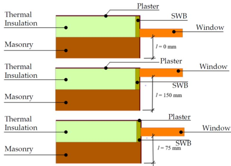
**Figure 8.** Schema of basic positions of the window frame in the section of the thermal insulation layer using SWB.
