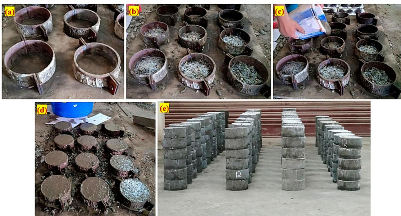
**Figure 7.** Casting procedure: (a) empty mold, (b) filling the mold with premixed fibers and coarse aggregate, (c) grout pouring process, (d) specimen appearance after casting, and (e) after demolding, where the specimens were left on the floor.
