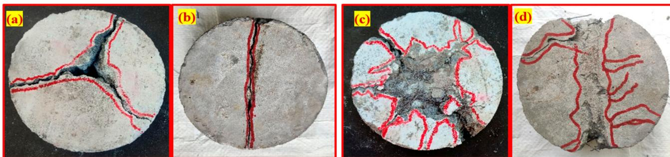
**Figure 14.** Comparison of failure pattern of specimens from ACI Committee 544 [38] and modified falling mass impact test: (a) ACI-nonfibrous, (b) modified-nonfibrous, (c) ACI- fibrous, (d) modified-fibrous.
