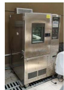
Figure 2. Simulation of daily temperature variations: (a) cyclic temperature regime; (b) programmable environmental chamber (Adapted from Ref. [32]).
