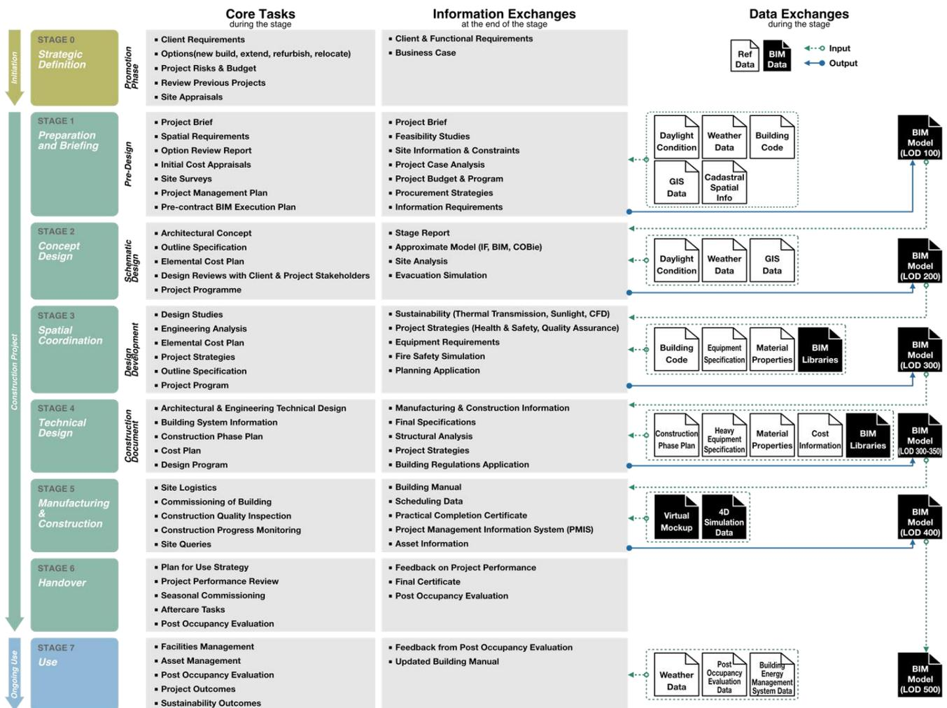
Figure 3. Data-centric construction process using referenced data and BIM-based data.
