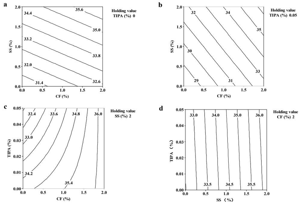
Figure 4. Effect of CF, TIPA and SS on the 3 d strength of cement mortars: (a) CF vs. SS (no TIPA), (b) CF vs. SS (0.05% TIPA), (c) CF vs. TIPA, (d) SS vs. TIPA.
