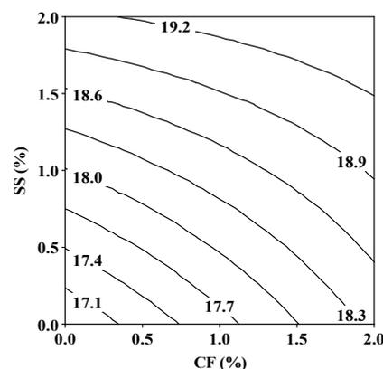
**Figure 3.** Effect of CF and SS on the 1 d strength of cement mortars.
