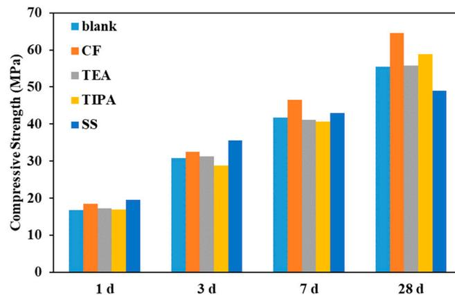
Figure 1. Effect of each admixture on the compressive strength of mortars (the content of each admixture refers to the high level in Table 3).
