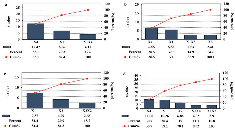
**Figure 2.** Pareto chart for the effectiveness of admixtures contributing to the strength development of mortars at different curing ages: (a) at 1 d, (b) at 3 d, (c) at 7 d, (d) at 28 d.
