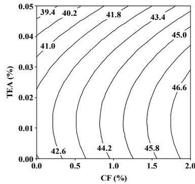
Figure 5. Effect of CF and TEA on the 7 d strength of cement mortars.
