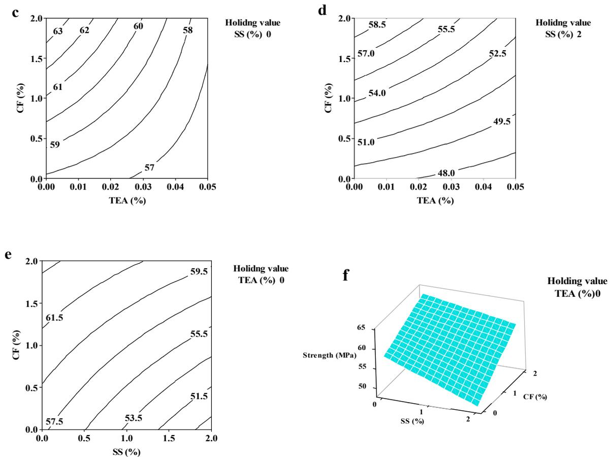
**Figure 6.** Effect of CF, TEA and SS on the 28 d strength of cement mortars: (a) SS vs. TEA (no CF), (b) SS vs. TEA (2% CF), (c) CF vs. TEA (no SS), (d) CF vs. TEA (2% SS), (e) CF vs. SS (2D contour plot), (f) CF vs. SS (3D contour plot).
