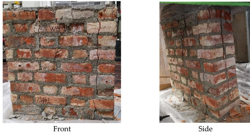
**Figure 7.** Crack patterns after the axial compression test.
