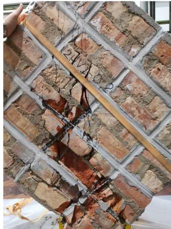
**Figure 12.** Local bending and shear damage of bars.
