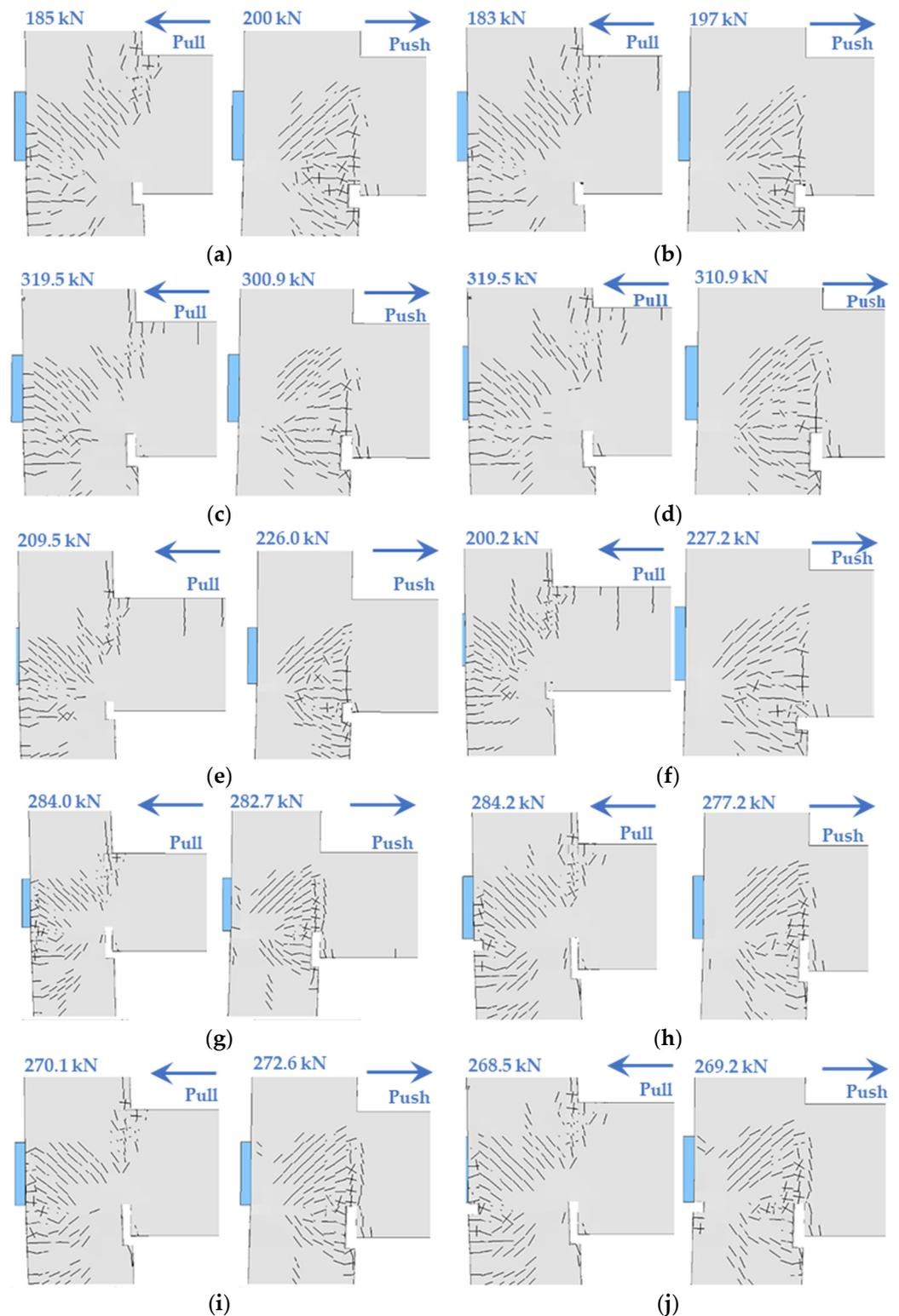
**Figure 18.** Crack and failure patterns of frame models: (a) H-C25; (b) L-C25; (c) HI-C40; (d) LI-C40; (e) H-C40; (f) L-C40; (g) HSQ-C25-T8; (h) LSQ-C25-T8; (i) HSQ-C25-T6; (j) LSQ-C25-T6.
