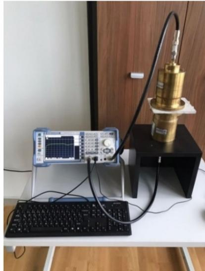
Figure 5. EM measurement system.
