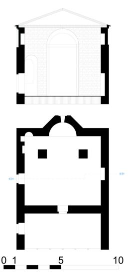
**Figure 10.** Plan layout and longitudinal section of the St Mary of Blachernae's church of Berat. Provision courtesy of Arch. Arsim Murseli, UBT University.
