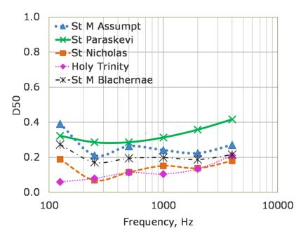
Figure 17. Measured results of definition (D<sub>50</sub>).
