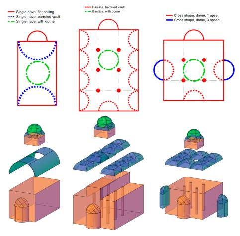
**Figure 1.** Drawn not to scale, different typologies of Byzantine churches. Plan layout (**above**) and 3D view (**below**).
