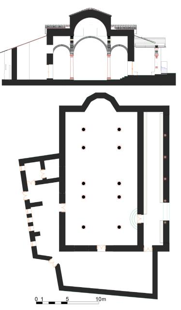
**Figure 2.** Plan layout and transversal section of St Mary Assumption's church. Provision courtesy of Arch. Arsim Murseli, UBT University, Pristina, Kosovo.
