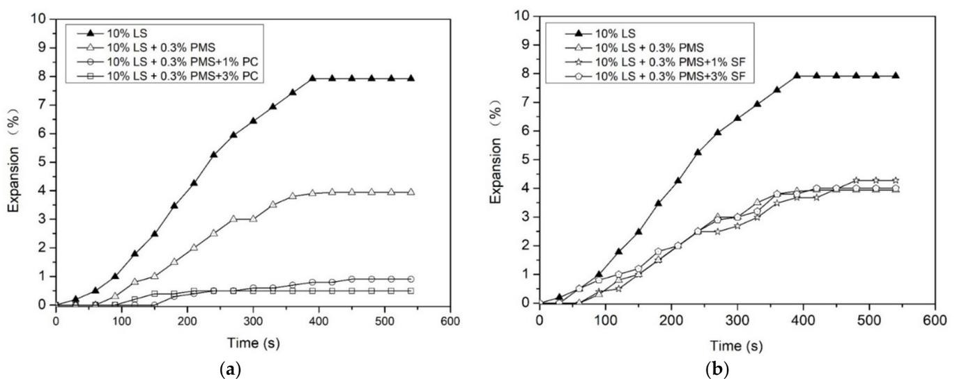
**Figure 7.** Expansion (before setting) of MAPC mortar samples with 10% limestone fines (LS) with or without defoaming treatment by the compound use of 0.3% polyether-modified silicone (PMS) defoamer and (a) Portland cement (PC); (b) silica fume (SF) at dosage of 1% and 3% (by weight of MAPC).
