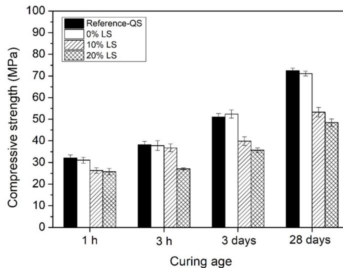
**Figure 4.** Compressive strength at different curing ages of 1 h, 3 h, 3 days, 28 days of MAPC mortar samples with quartz sand (Reference-QS) and limestone fines (LS) at different content of 0%, 10%, 20%.
