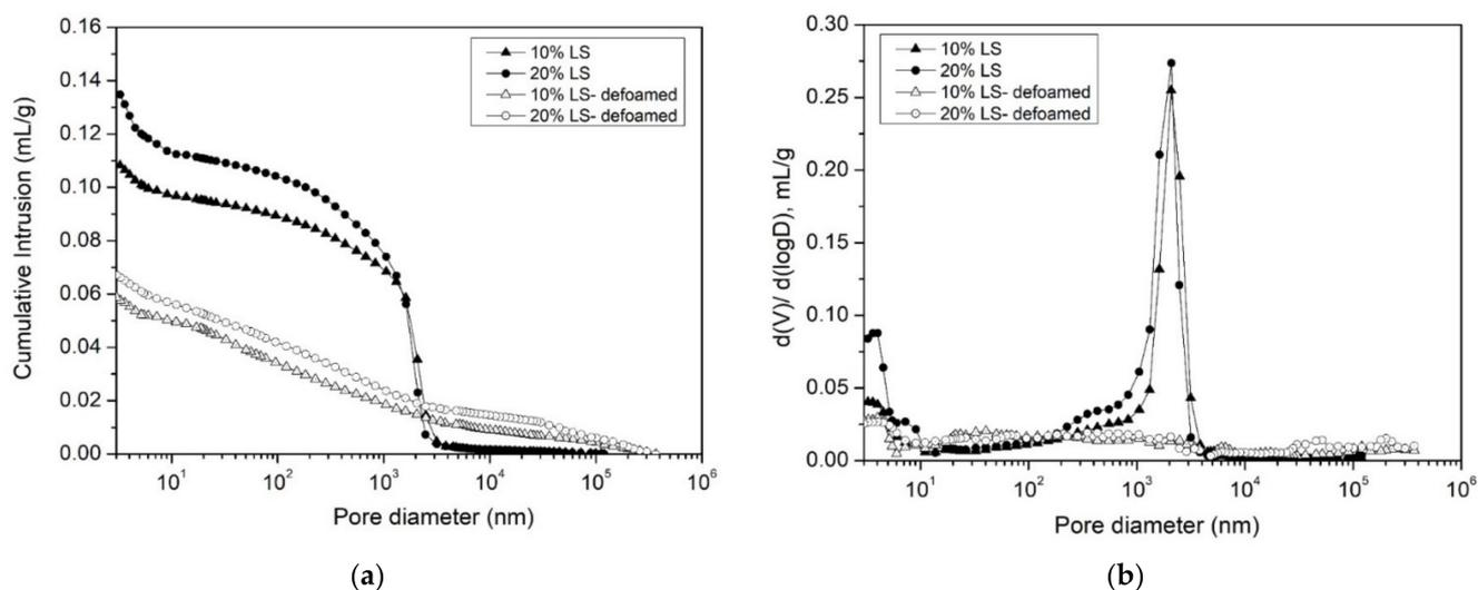
**Figure 10.** Mercury intrusion porosimetry (MIP) results on MAPC mortar samples with limestone fines (LS) at content of 10% and 20% with or without defoaming treatment by the compound use of 0.3% polyether modified silicone (PMS) defoamer and 1% Portland cement (PC): (a) Cumulative intrusion; (b) differential pore-size distribution.
