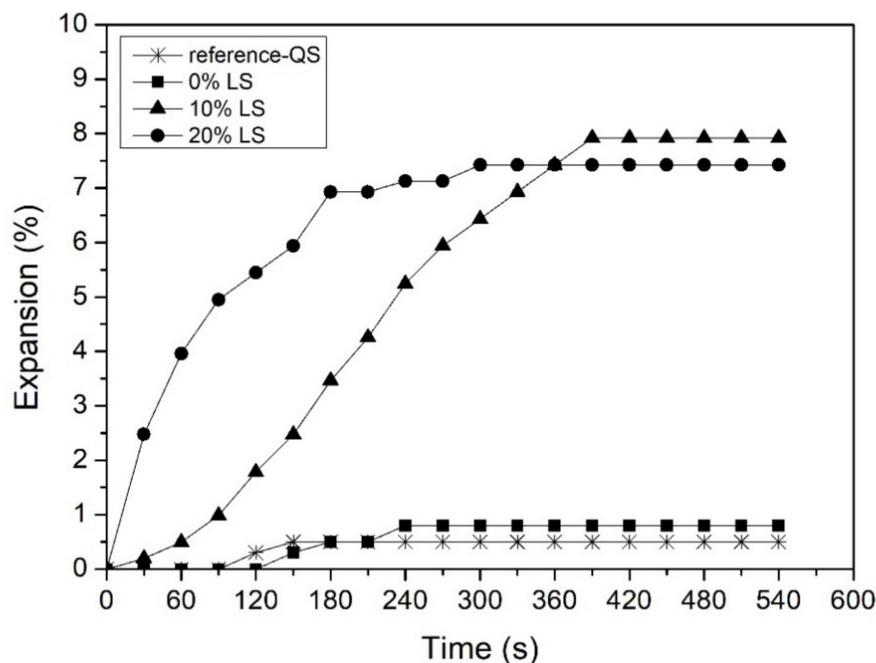
**Figure 3.** Expansion (before setting) of MAPC mortar samples with limestone fines (LS) at different dosage of 0%, 10%, 20% (by weight of MAPC).
