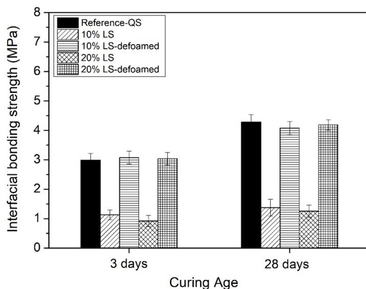
**Figure 9.** Interfacial bonding strength (at curing age of 3 days, 28 days) of MAPC mortar samples containing limestone fines (at content of 10% and 20%) with or without defoaming treatment by the compound use of 0.3% polyether modified silicone (PMS) defoamer and 1% Portland cement (PC).
