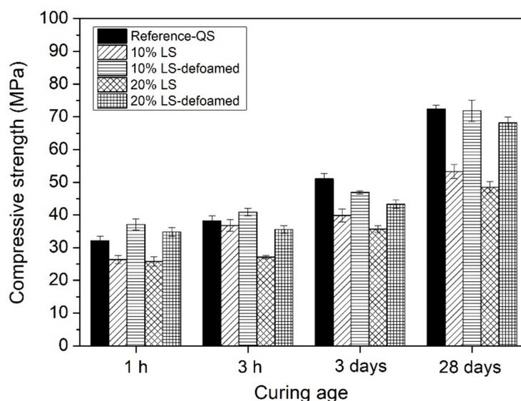
**Figure 8.** Compressive strength (at curing age of 1 h, 3 h, 3 days, 28 days) of MAPC mortar samples containing limestone fines (at content of 10% and 20%) with or without defoaming treatment by the compound use of 0.3% polyether modified silicone (PMS) defoamer and 1% Portland cement (PC).
