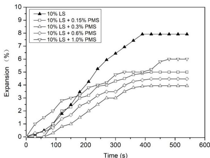
**Figure 6.** Expansion (before setting) of MAPC mortar samples with 10% limestone fines (LS) with or without defoaming treatment by polyether modified silicone (PMS) defoamer at different dosage of 0.15%, 0.3%, 0.6%, and 1% (by weight of MAPC).
