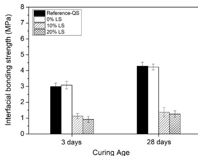
**Figure 5.** Interfacial bonding strength at different curing ages of 3 days, 28 days of MAPC mortar samples with quartz sand (Reference-QS) and limestone fines (LS) at different contents of 0%, 10%, 20%.
