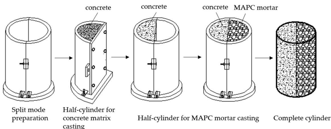
**Figure 2.** Sample preparation for test on interfacial bonding strength of MAPC mortar with ordinary concrete matrix.
