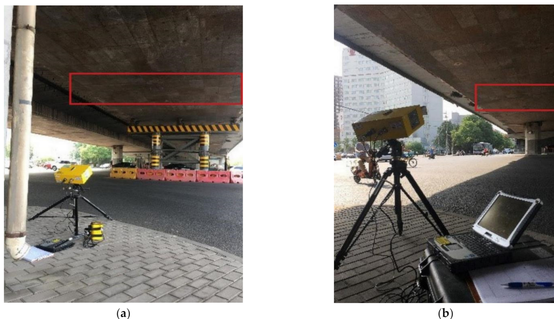
Figure 4. Layout of IBIS-S to obtain dynamic deflection. (a) Layout of IBIS-S of RSB and (b) layout of IBIS-S of LSB.
