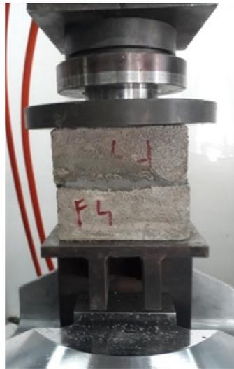
**Figure 5.** Setup for compression tests.
