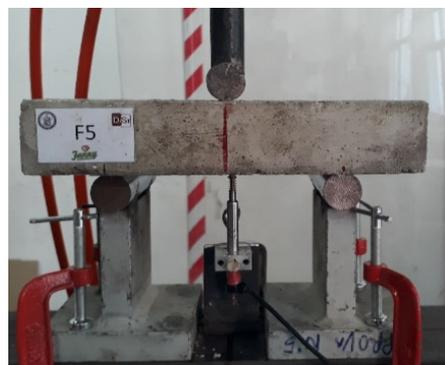
**Figure 4.** Setup for the three-points bending test.
