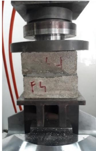
**Figure 5.** Setup for compression tests.
