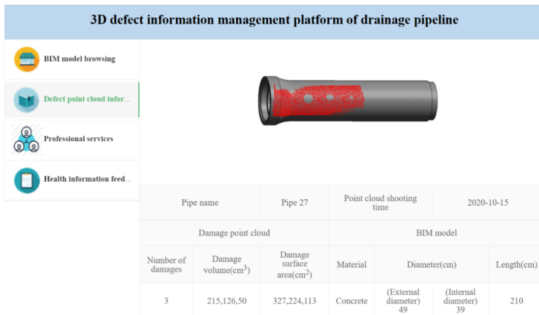
Figure 14. Defect point cloud information.
