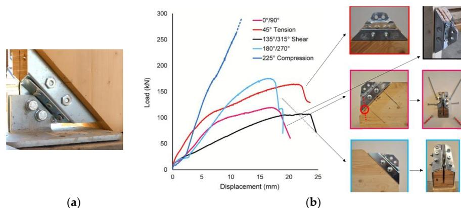
**Figure 6.** X-RAD system: (a) HD connector (photo credit: Rothoblaas, reprinted with permission); (b) force–displacement curves and failure modes (photo credit: Andrea Polastri, reprinted with permission).
