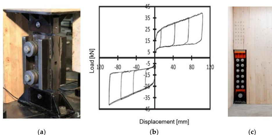
**Figure 9.** RSF HD: (a) close-up view; (b) force–displacement (photo credit: Ashkan Hashemi, reprinted with permission); (c) commercial application (photo credit: Fast + Epp, reprinted with permission).
