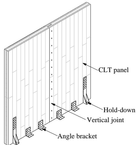
**Figure 2.** CLT shear wall connections (schematic produced by David Owolabi (UBC student, reprinted with permission)).
