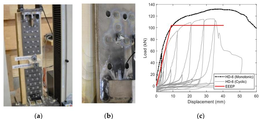
**Figure 11.** (a) HD with STS; (b) failure mode (photo credit: Thomas Tannert); (c) force–displacement curves.
