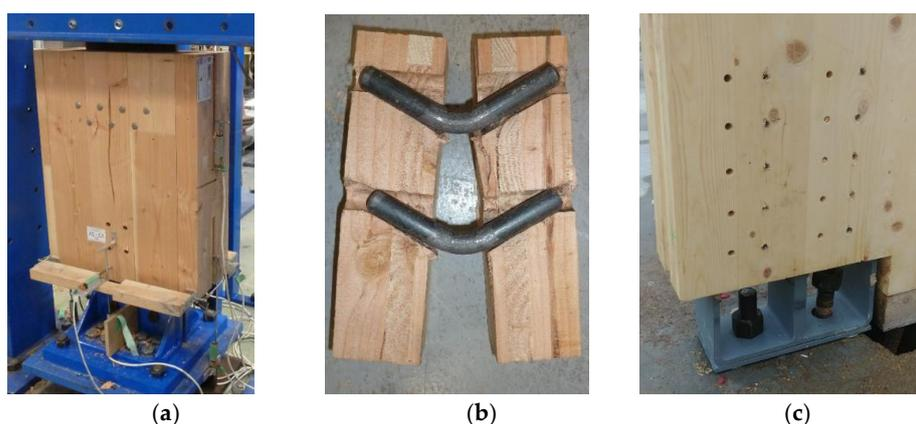
**Figure 4.** Dowelled slotted-in steel plates: (a) HD test setup; (b) ductile steel yielding and wood crushing failure modes (photo credit: (a,b) Justin Brown; (c) Fast + Epp, reprinted with permission).
