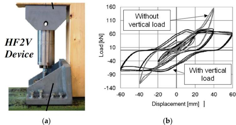
**Figure 10.** Damper-based HD: (a) close-up view of the damper device (photo credit: Geoffrey Rodgers, reprinted with permission); (b) typical load–displacement curve.
