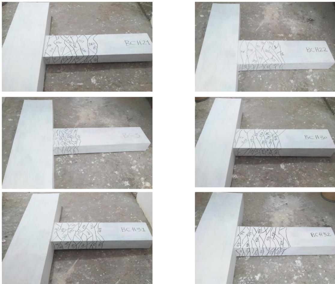
Figure 13. Crack pattern of tested specimens.
