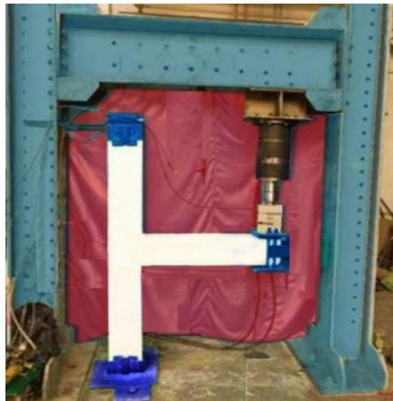
**Figure 9.** Test setup for exterior beam-column connection.
