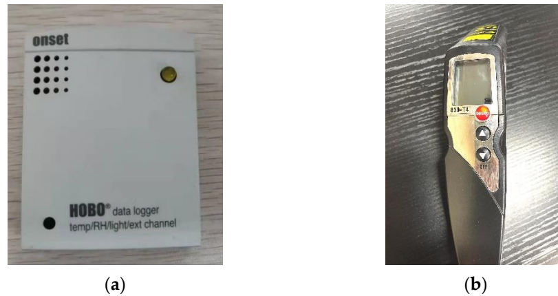
Figure 4. Experimental instruments: (a) HOBO U12-012; (b) Testo 830-T4.
