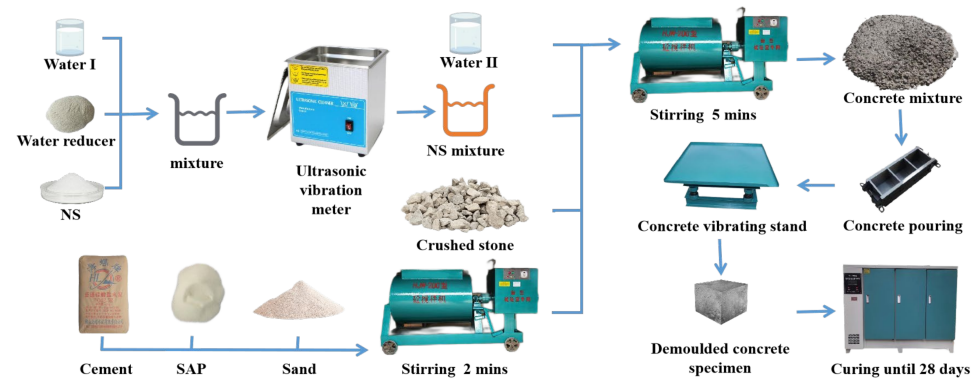
Figure 1. Preparation procedure and process of concrete specimens.
