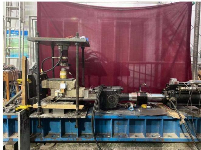
Figure 12. Test setup of mortar joint shear.
