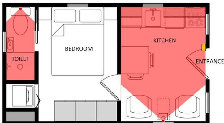
**Figure 16.** The third configuration of the home sensors network of Case Study 2.
