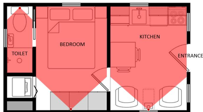
**Figure 14.** The first configuration of the home sensors network of Case Study 2.
