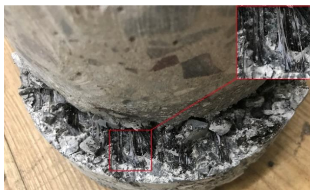
Figure 11. The interface of fracture after the shearing test.
