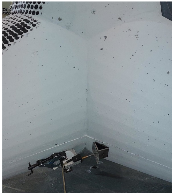
Figure 4. Additional inductive-displacement-sensor for measuring the crack width (specimen L22033_2_2).
