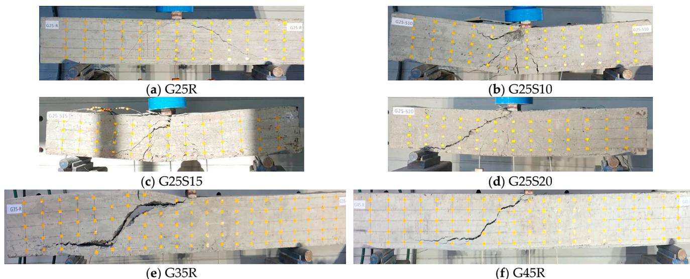
**Figure 4.** Cracking patterns and failure modes of the tested beams.
