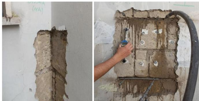
Figure 12. Corner detail and flat jack test of masonry walls made of Neapolitan yellow tuff stones.
