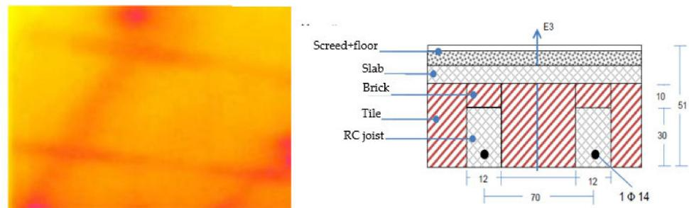
Figure 10. First level ribbed floor.
