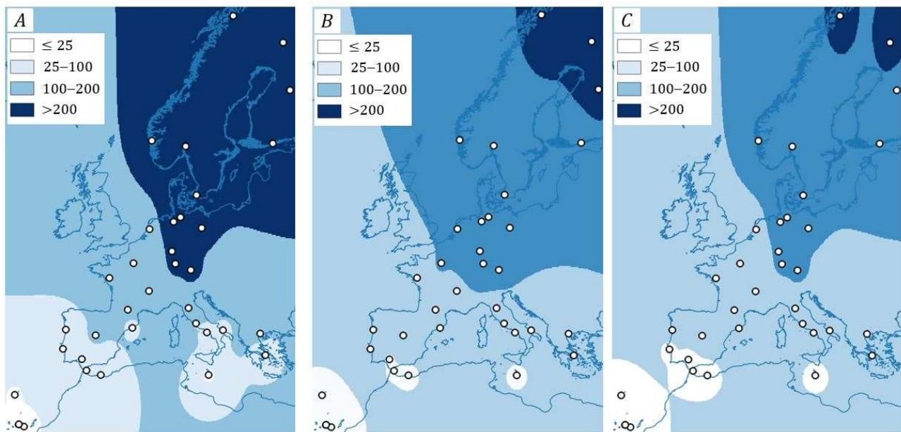
**Figure 4.** Heating demand intervals ( $\text{kWh}/\text{m}^2/\text{year}$ ) interpolated by IDW for the reference building with double-glazed windows of 4 + 12 + 6 mm and without insulation in the envelope (A), with insulation thicknesses of 40 mm (B) and with thicknesses of 80 mm insulation (C).
