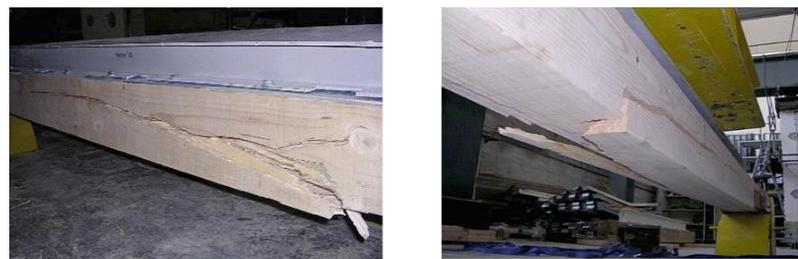
(a) Experimental failure mode.
