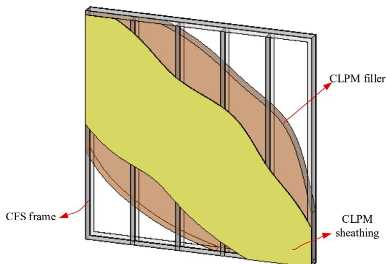
**Figure 1.** Configurations of CFS-CLPM composite walls.
