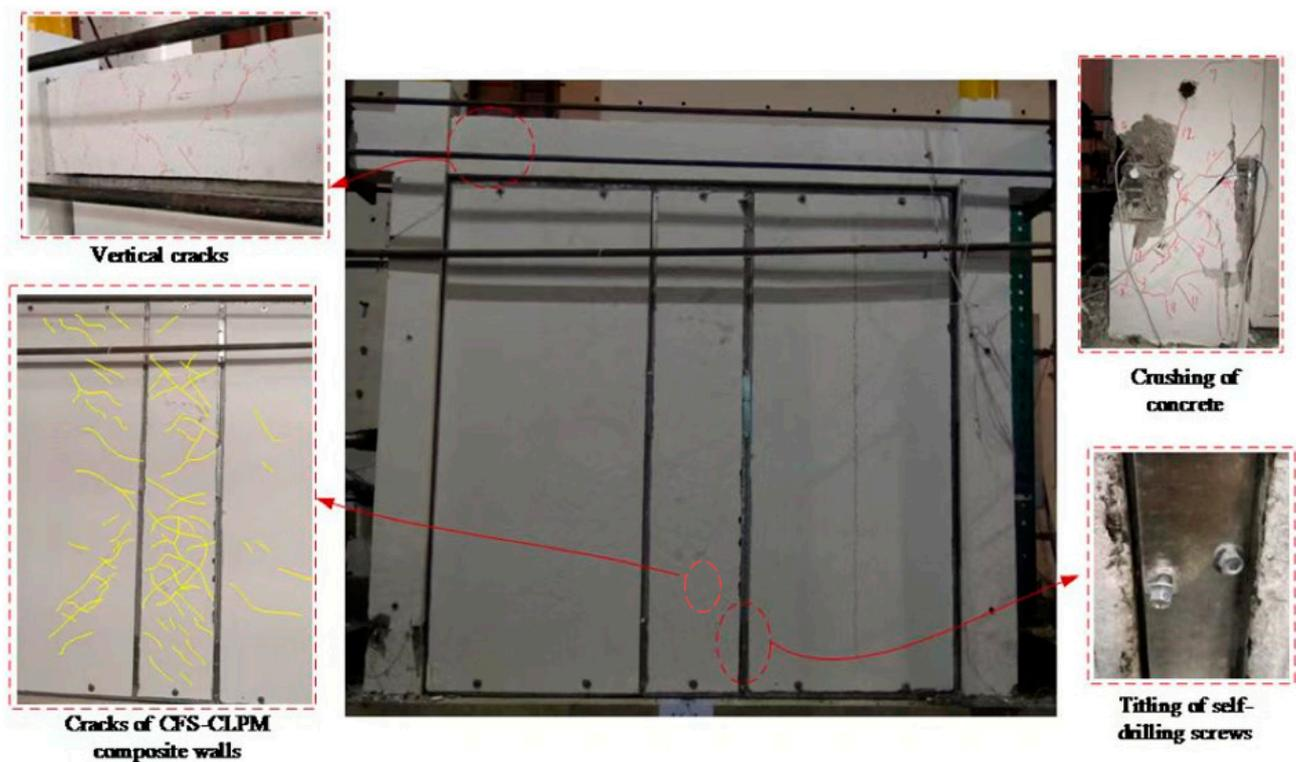
Figure 10. Failure modes of specimen PCFW.
