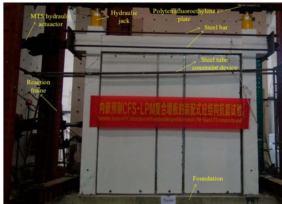
Figure 6. Test set up.
