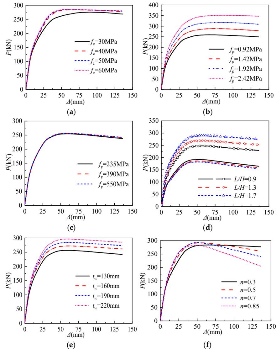
**Figure 21.** Influence of different parameters on lateral response of PC frame infilled with CFS-CLPM composite walls: (a) Compressive strength of concrete; (b) Compressive strength of CLPM; (c) Strength of cold-formed steel; (d) Span to height ratio; (e) Thickness of CFS composite walls; (f) Axial load ratio.
