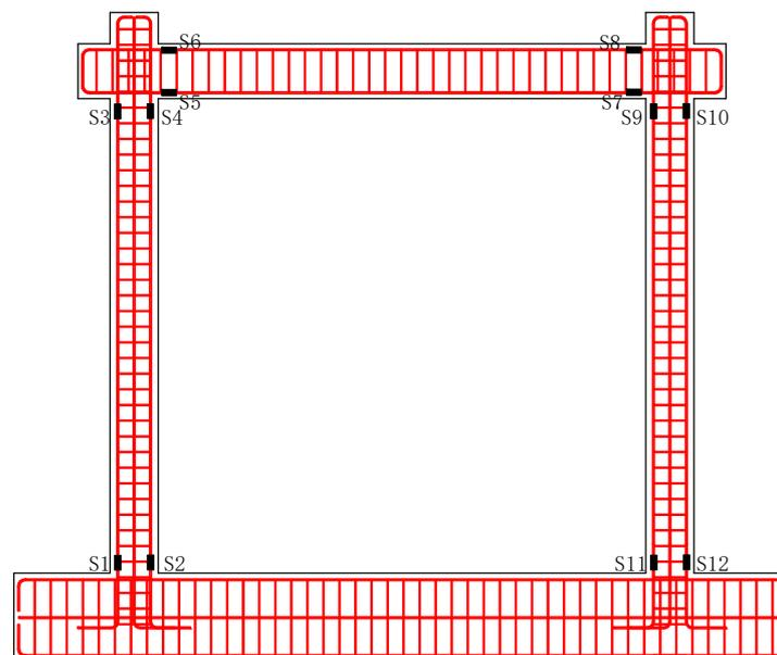
Figure 7. Strain gauges arrangement on the PC frame.
