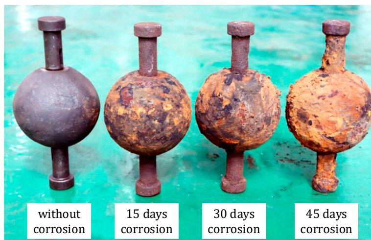
Figure 5. Corroded bolt-sphere connections.
