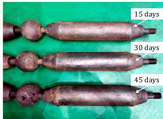
**Figure 6.** Corroded bolt-sphere joints with members.
