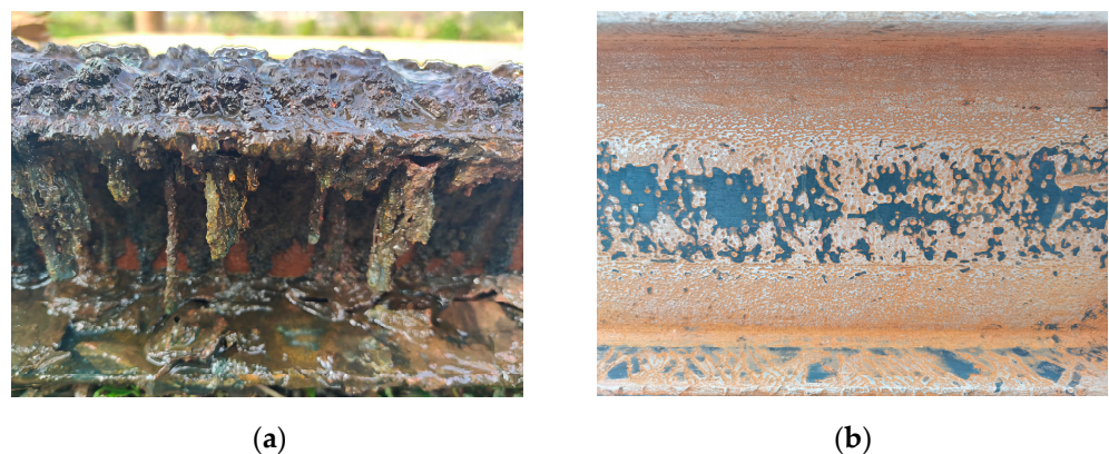
Figure 3. Specimens after corrosion: (a) Corrosion products; (b) Surface morphology of the specimens.
