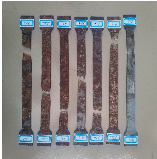
Figure 8. Failure mode of the tensile specimens.
