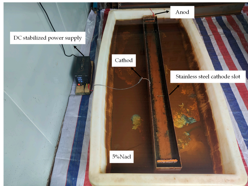
Figure 2. Electrochemical corrosion test.
