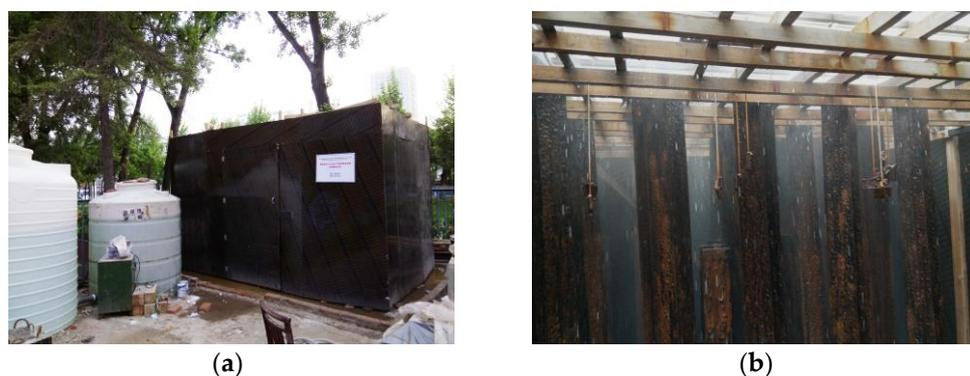
**Figure 1.** Accelerated corrosion test of H-beams: (a) general view of the test platform and (b) schematic diagram of internal sprinkler.
