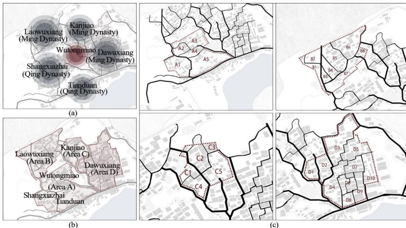
**Figure 4.** (a) The layout of the Wutongmiao, Laowuxiang, Kanjiao, Dawuxiang, Tianduan, and Shangzhai housing clusters; (b) class I fire-protection group zoning; and (c) secondary fire-protection zoning.
