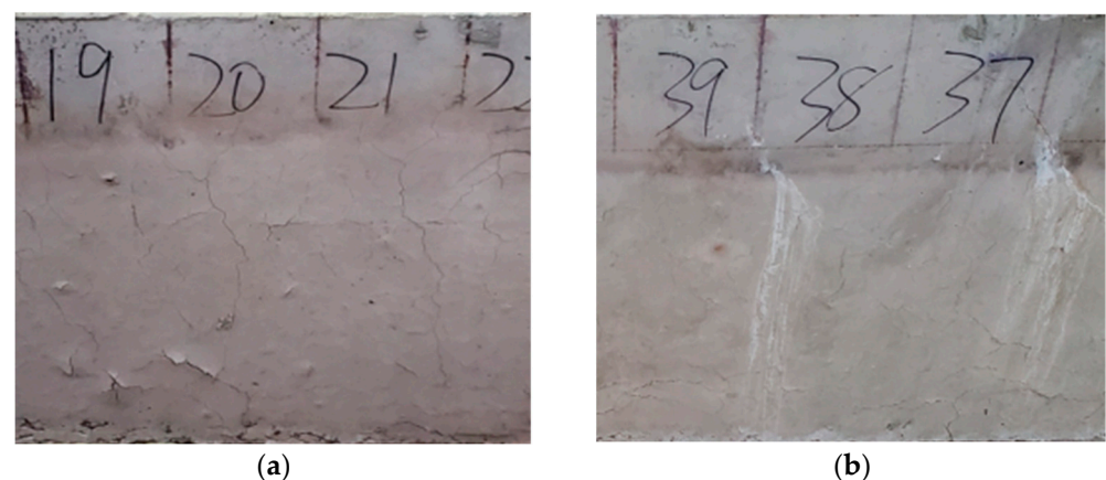
Figure 6. Water stain drawing of beam side: (a) ITSC beam; (b) NSC beam.
