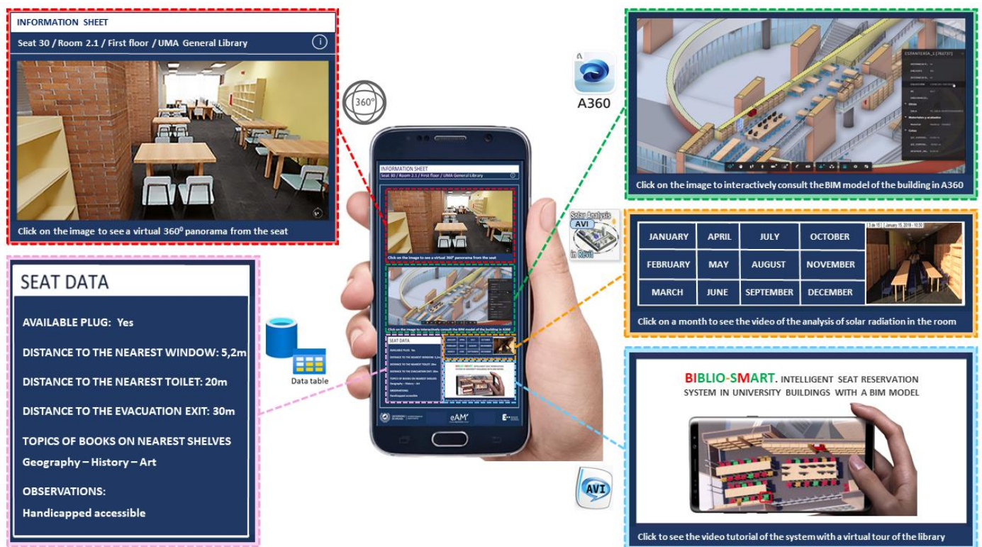
Figure 10. Biblio-Smart app interface designed to consult information of interest for the reservation from BIM model data, with its expanded options and icons of the file format or tool used.
