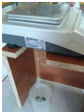
Figure 3. Apparatus for the immersed apparent mass determination.
