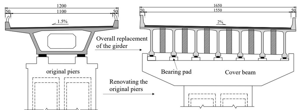
Figure 4. Overall replacement of the girder (unit: cm).
