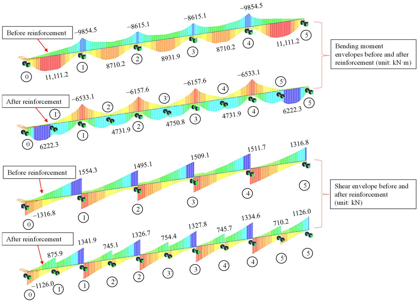
Figure 9. Bending moment and shear envelopes before and after reinforcement.
