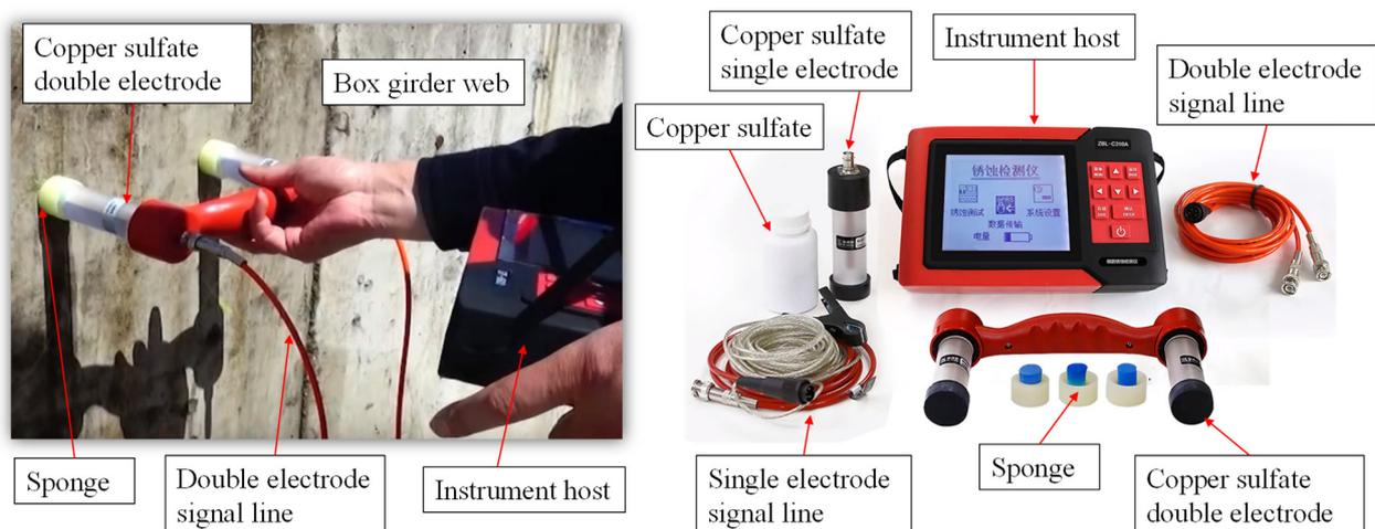
**Figure 3.** Corrosion potential testing of steel bars in concrete.
