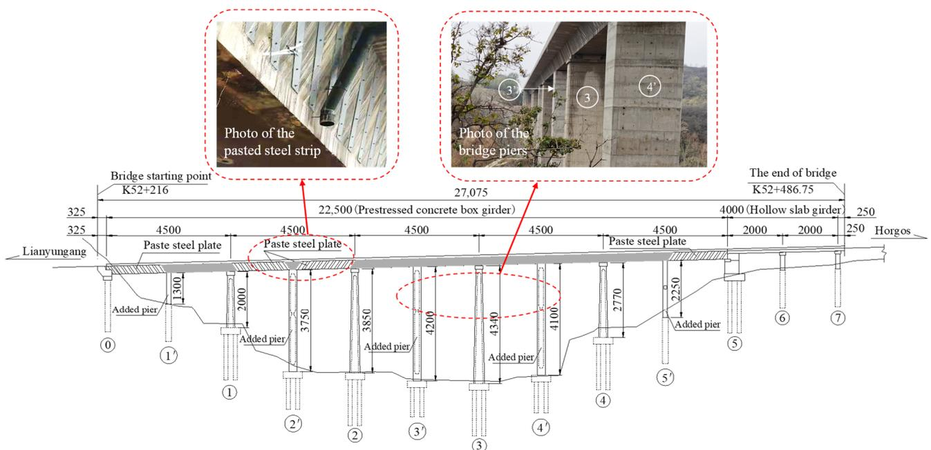
**Figure 6.** Reinforcement schematic of Scheme 2 (unit: cm).
