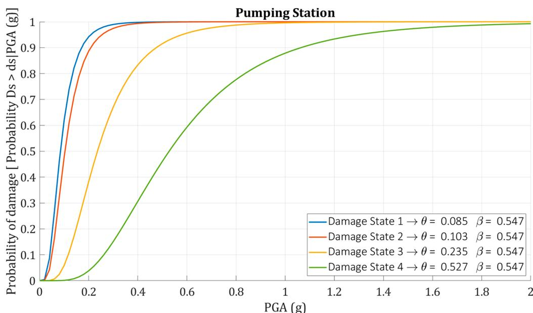
**Figure 2.** The exclusive fragility curves that were derived for an oil pumping station (based on [51]).
