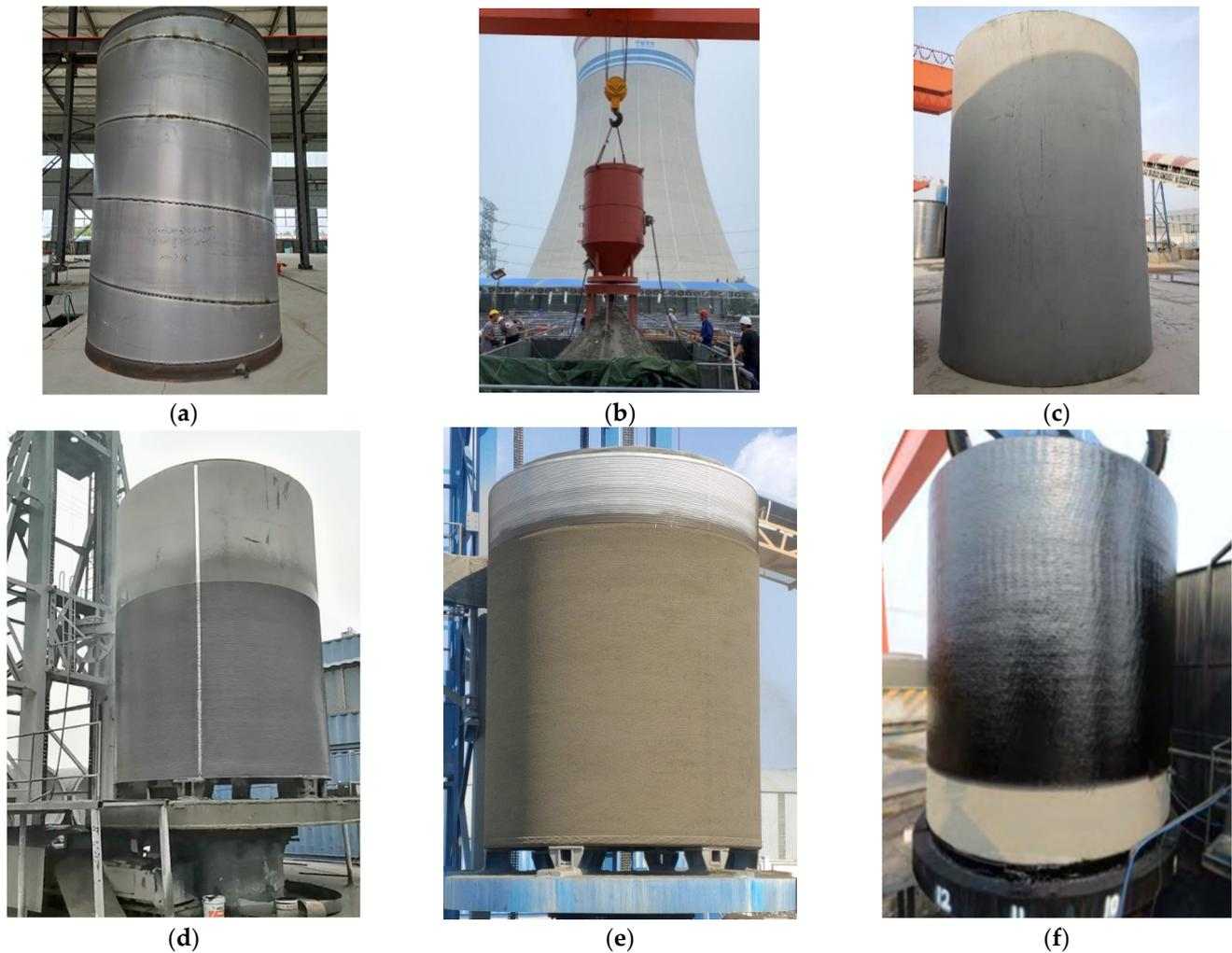
**Figure 3.** The manufacture process of PCCP: (a) Welded steel cylinder; (b) Pouring of concrete; (c) Concrete core; (d) Wrapping of prestressed steel wire; (e) Roll shooting of protective mortar; (f) Anti-corrosion coating.
