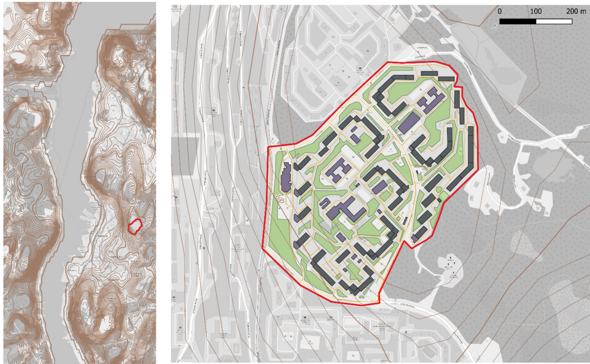
Figure 19. Design project of neighborhood 403, Murmansk, including the topographic contour and the prevailing wind direction.
