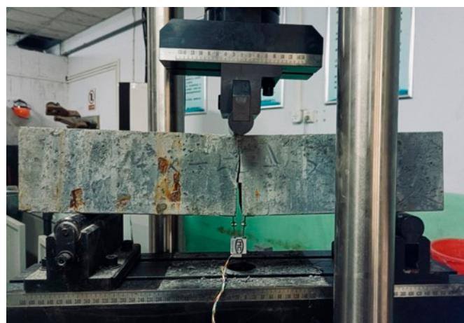
**Figure 2.** The three-point bending test process.
