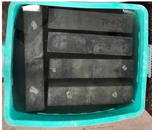
**Figure 3.** The specimens soaking in sodium sulfate solution.
