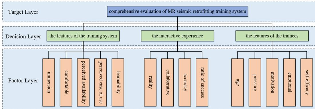
Figure 6. The AHP evaluation indicator system of the MR seismic retrofitting training system.
