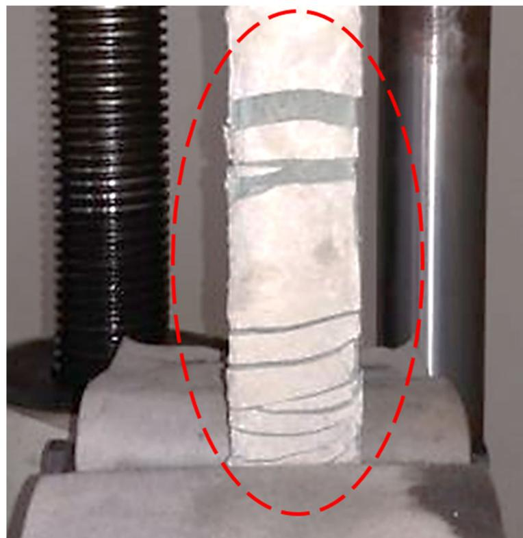
**Figure 19.** Crack pattern in tested TRM specimen (TRM2).
