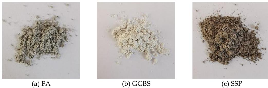
**Figure 1.** The three mineral admixtures used in the experiment.
