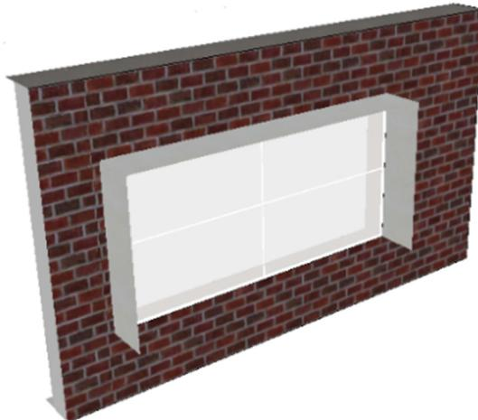
**Figure 10.** The best-performing external shading option of overhang and side fins with 0.8 m projection for the west façade existing windows.
